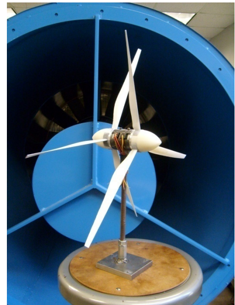
Figure 1. Counter-Rotating Wind Turbine Test Apparatus
