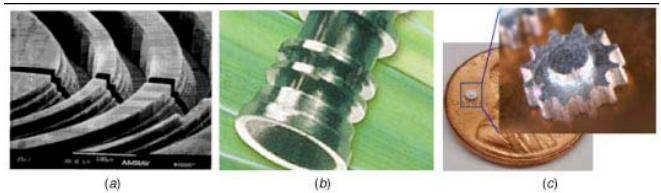
Figure 1. System Layout a) Micromilled trenches with stepped walls, b) neurovascular device component, c) microgear
