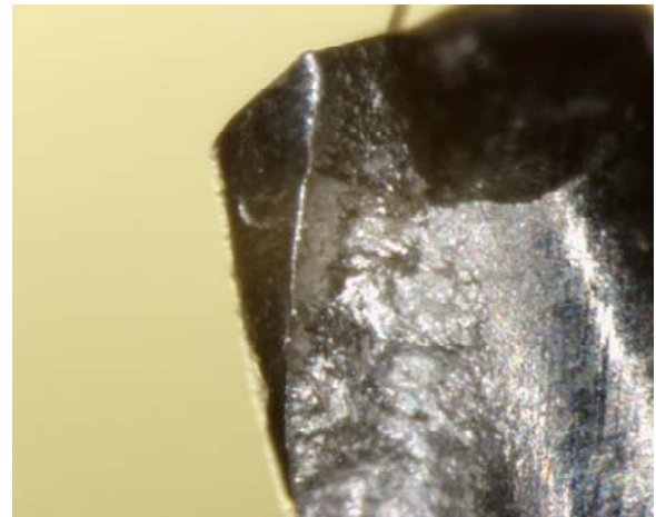
Figure 8. Wear of micromill working at v_c=130 m/min
