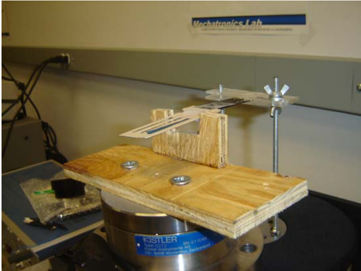
Fig. 5. One of the tested wings with three slots on the dynamometer
