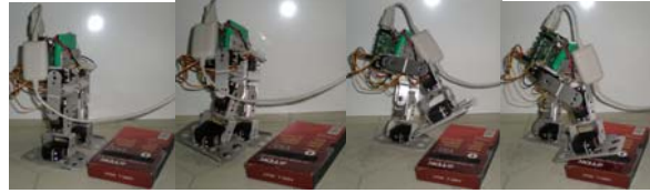
Figure 14. Climbing up stairs.
