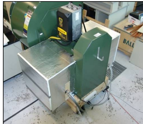
Figure 10. Insulated box for cooling electrical motor
